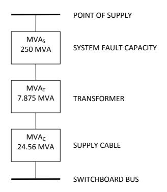
The total Fault MVA for the system will be:
