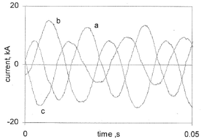
Fig. 8 Arcing Currents at 208V, 9.9kA - With Barrier
