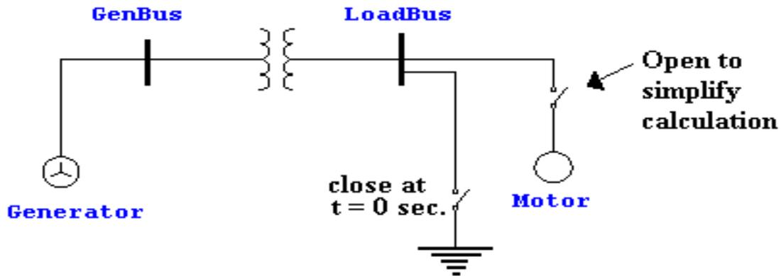
Equivalent Impedance Diagram
