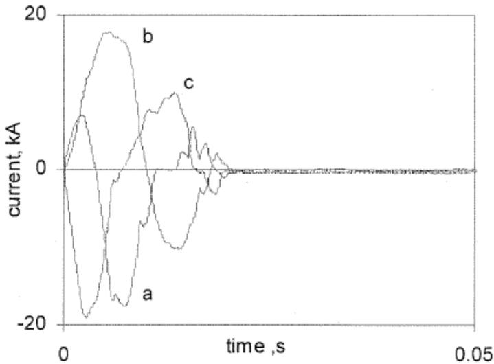
Fig. 6 Arcing Currents at 250V, 13kA - No Barrier .
