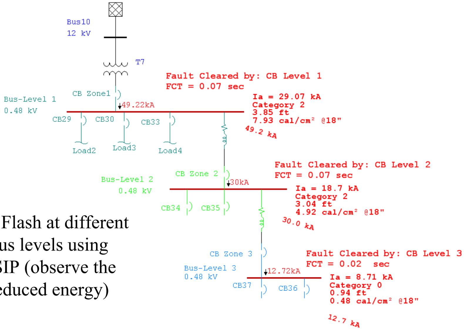
Arc Flash at different bus levels using ZSIP (observe the reduced energy)
