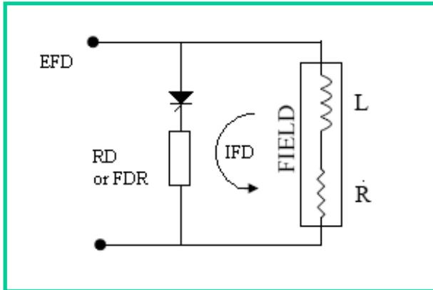
A Field Discharge Resistor (FDR) is added along with the generator Time Constant ( $T'_{do}$ )
