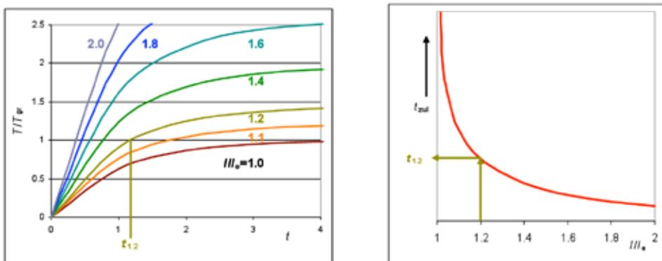
a) Heating at loading with rated current ( $1.0 \cdot I_n$ ) and at various overcurrent levels ( $1.2 \cdot, 1.5 \cdot, 1.7 \cdot, 2 \cdot I_n$ )
