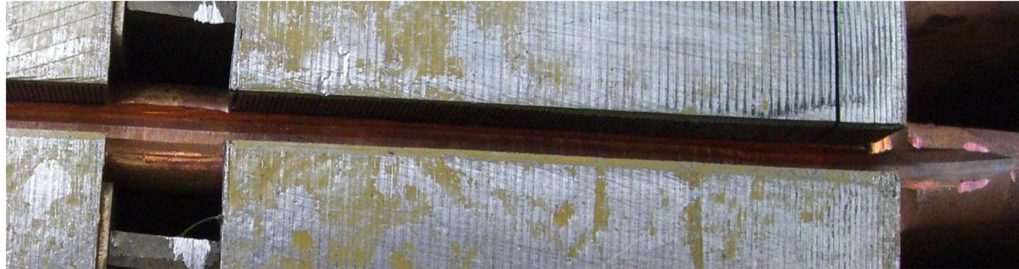
Rotor bars can be swaged for a tight fit in the slot.
