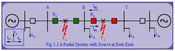
In contrast, there can be situations where for the purpose of selectivity, phase angle information (always relative to a reference phasor) may be required. Fig 2.2 shows such a case for a radial system with source at both ends. Consequently, fault is fed from both the ends of the feeder. To interrupt the fault current, relays at both ends of the feeder are required.
