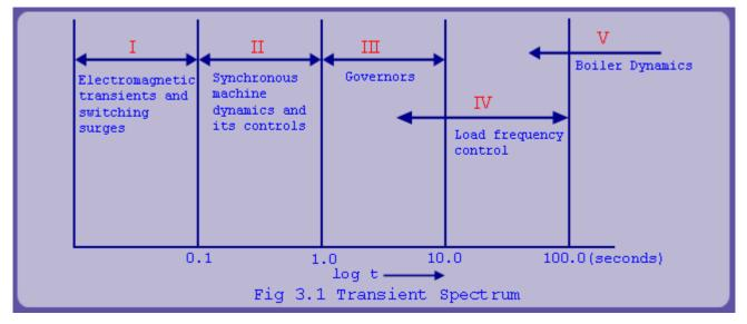
Figure 3.1 shows the various time scales involved in modelling system dynamics. The dynamics involved in switching, lightening, load rejection etc have a high frequency component which die down quickly. In analysis of such dynamics, differential equations associated with inductances and capacitances of transmission lines have to be modelled. Such analysis is restricted to a few cycles. It is done by Electromagnetic Transient Program (EMTP).
