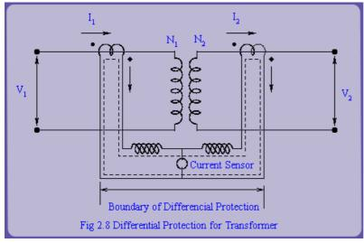
Differential protection for detecting faults is an attractive option when both ends of the apparatus are physically located near each other. e.g. on a transformer, a generator or a bus bar.
