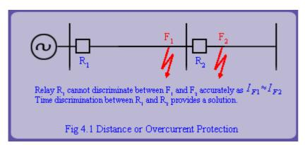
Like sensitivity, selectivity also implies an ability to discriminate. A relay should not confuse some peculiarities of an apparatus with a fault. For example, transformer when energized can draw up to 20 times rated current (inrush current) which can confuse, both overcurrent and transformer differential protection. Typically, inrush currents are characterized by large second harmonic content.
