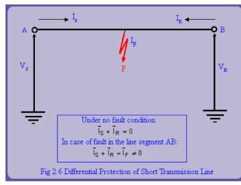
Differential protection is based on the fact that any fault within an electrical equipment would cause the current entering it, to be different, from the current leaving it. Thus by comparing the two currents either in magnitude or in phase or both we can determine a fault and issue a trip decision if the difference exceeds a predetermined set value.
