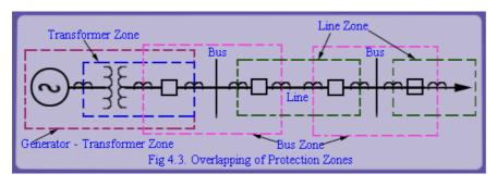
A relay's zone of protection is a region defined by relay's jurisdiction (see fig 4.3). It is shown by demarcating the boundary. This demarcation for differential protection is quite crisp and is defined by CT's location. On the other hand, such boundaries for overcurrent and distance relays are not very crisp. It is essential that primary
