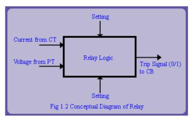
Formally, a relay is a logical element which processes the inputs (mostly voltages and currents) from the system/apparatus and issues a trip decision if a fault within the relay's jurisdiction is detected. A conceptual diagram of relay is shown in fig 1.2.
