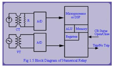
The block diagram of a numerical relay is shown in fig 1.5.
