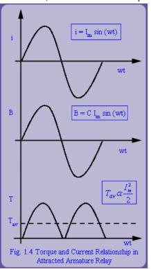
When the deflection exceeds a preset value, the relay contacts closes and a trip decision is issued. Electromechanical relays are known for their ruggedness and immunity to Electromagnetic Interference (EMI).
