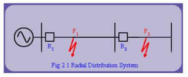
This scheme is based on the intuition that, faults typically short circuits, lead to currents much above the load current. We can call them as overcurrents. Over current relaying and fuse protection uses the principle that when the current exceeds a predetermined value, it indicates presence of a fault (short circuit). This protection scheme finds usage in radial distribution systems with a single source. It is quite simple to implement.
