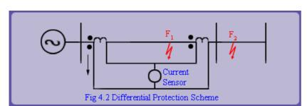
However with a differential protection the CT location provides 'crisp' demarcation of zone of protection of CT (see fig 4.2). The fault  $F_1$  is in the relay's zone of protection, but fault  $F_2$ is not in its jurisdiction. Because differential protection scheme do not require time discrimination to improve selectivity, they are essentially fast.
