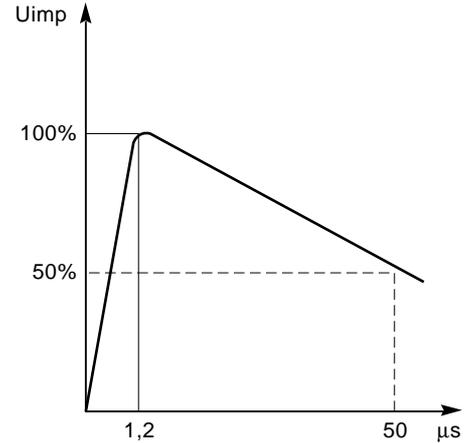
**fig. 10:** impulse wave for industrial circuit breakers 1.2/50  $\mu\text{s}$ .
