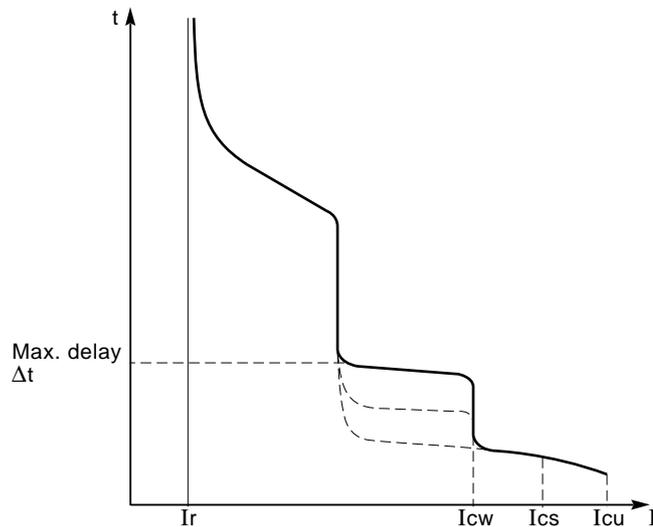
**fig. 4:** Additional test for category B circuit breakers.
