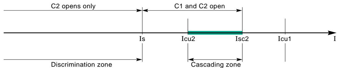
**fig. 7:** The principle of cascading between 2 circuit breakers, breaker C2 whose breaking capacity  $I_{cu2}$  is less than the three-phase short-circuit current at its terminals ( $I_{sc2}$ ), is protected or assisted by breaker C1.
