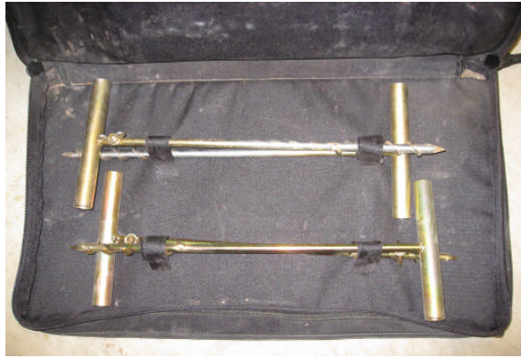
Fig. 15 - T-Handle, Factory-Made Test Probes in a kit of four
