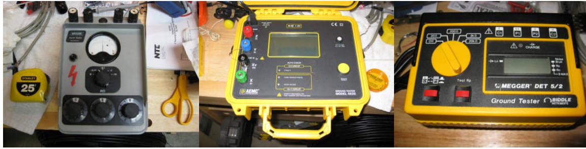
Fig. 3 – Typical Test Sets (l-r: Biddle “Megger” 240241, AEMC 4630, Biddle DET5/2)
