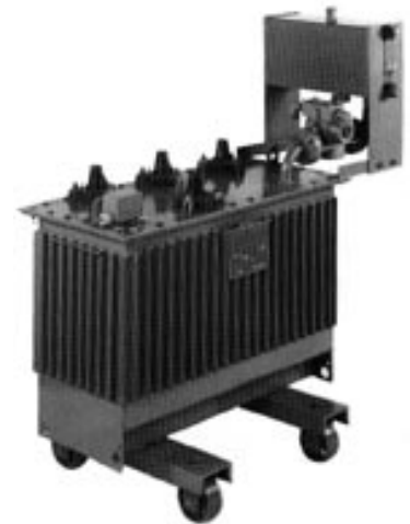
fig. 1 : a zigzag or neutral point coil provides an earth fault current limiting reactor.
